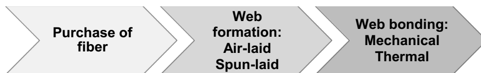
Fig. 4.8: Different steps of manufacturing non-woven fabrics
